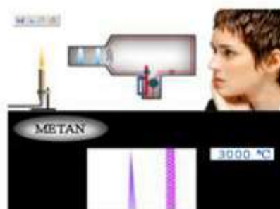
1- rasm. “Optik pirometr yordamida gazlarning yonish alangasini aniqlash” animatsion tajriba ishidan fragment
