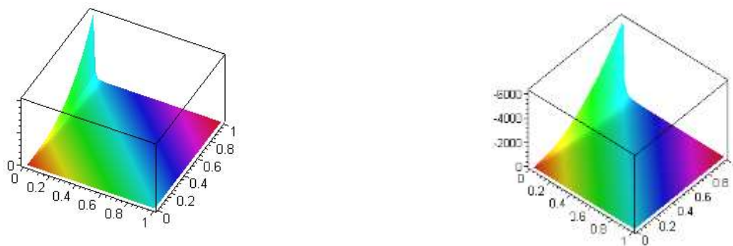
Fig.5. The space and time evolution of the normalised current density j(x,t) for n = 1, 3 .
